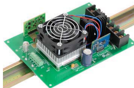
Assembled EVAL117 with PAD117A mounted. Shown with optional PAD125, PAD131 and DIN rail mounting.
